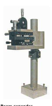
**Beam expander**Beam expander for mouting microscope objectives and pinhole. Easily adjustable both in heigth as sideways.
