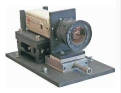
**Shift camera**Used on a lineair track for grabbing sequences of photographs for MPGH holograms
